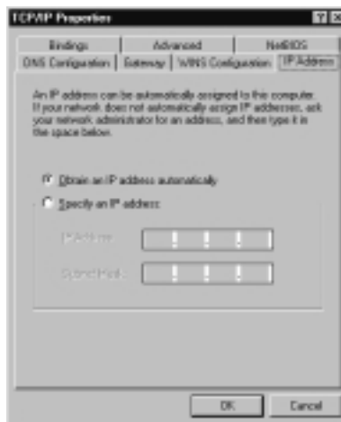
Figure 9.5 TCP/IP Properties Window with Dynamic IP Address
