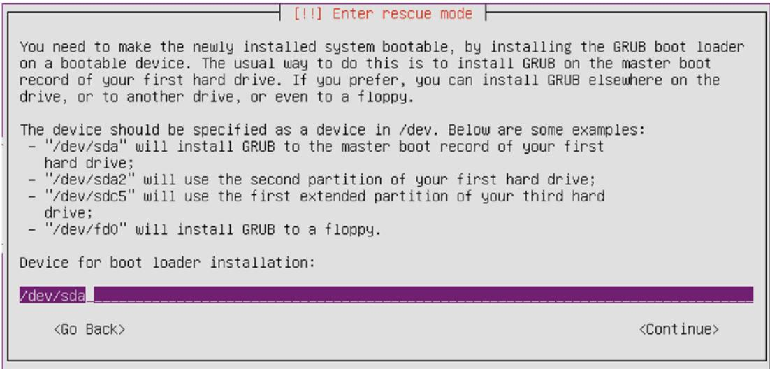
**Figure 9-10.** Re-installing the GRUB boot loader
